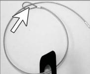
3. Depress cable release button 3. and hold down.
