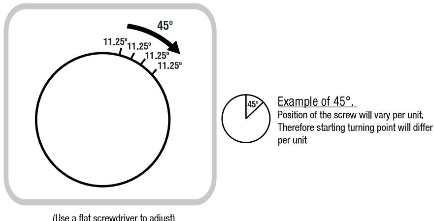
**NOTE:** If the compressor runs continuously for more than 1 hour turn the screw counterclockwise a few degrees (0-45°) until the compressor stops (allow 10 minutes timeframe after each adjustment for the compressor to stop).
