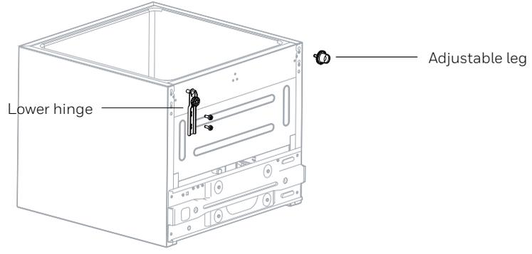
**06 06** Put the door on lower hinge vertically, then install the upper hinge by fitting screws and the hinge cover. Cover the hole caps on upper right side.
