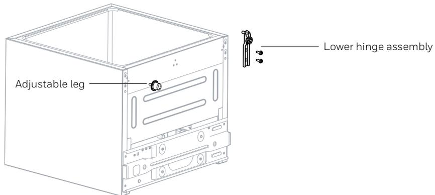
**05** Install the lower hinge and adjustable leg on lower left side of cabinet and lower right side respectively;
