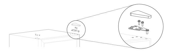
Put the glass door on the lower hinge, install the door axle sleeve back and then install the upper hinge. Align the door with the cabinet and check the tightness of gasket.
