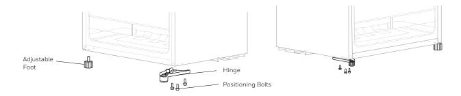
Remove the adjustable foot, positioning bolts and lower hinge, then exchange the parts of right and left sides and later use the reverse method to install the adjustable foot and positioning bolts.
