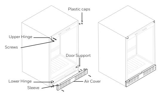
Remove the sleeve and the hole cap of the door, and change their positions. Remove the door stopper, screw and lower shaft sleeve, and then install them into the left lower corner of the door.
