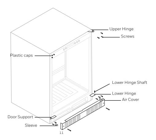
Take out the left upper hinge, and secure it on the left upper corner with a screw. Install the hole caps onto the right upper corner. Remove the lower hinge shaft and install it into the hole on the left side. Then secure the lower hinge onto the left lower corner with a screw. Install the door support onto the right lower corner with a screw. Then, install the air cover by using a screw and a sleeve on the lower side of the cabinet.
