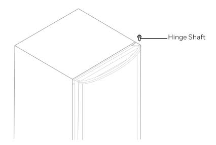
Remove 3 screws from the upper hinge on the right side then remove the upper hinge. Remove 3 plastic caps on the left side. From the air cover, remove screws and the sleeve. Then remove the air cover. Remove the door support, and remove 3 screws from the lower hinge. Remove the lower hinge and the lower hinge shaft.
