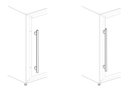
Use the allen wrench to fix the handle, making sure the screw hole is downward.
