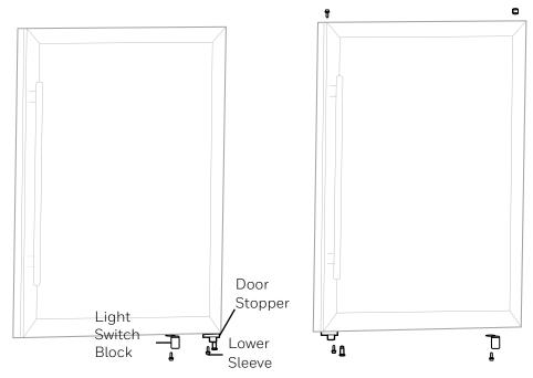
**02** Rotate the door assembly 180 degrees, exchange the position of the upper sleeve and the shaft plug, then move the foor stopper and the lower sleeve from the lower right to the lower left.
