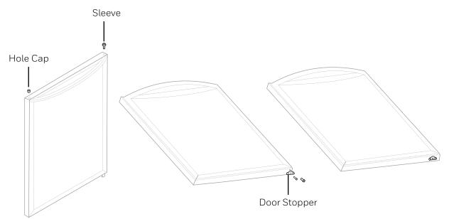
Install the door, and fix the upper hinge shaft.
