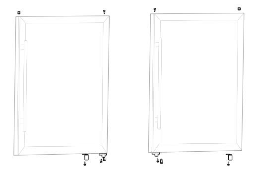
**03** Assemble the sleeves, the shaft hole cap, the stopper and the switch block.
